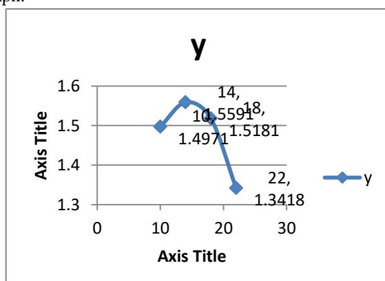
Calculation of optimum moisture content and maximum dry density for 5% ESP&25% FLY ASH
