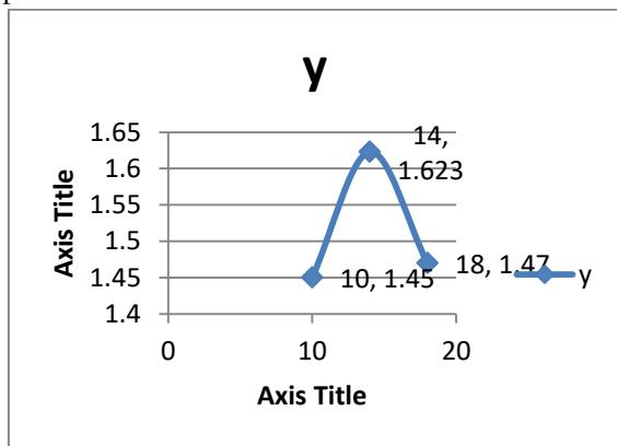
Calculation of optimum moisture content and maximum dry density for 5% ESP&30% FLY ASH
