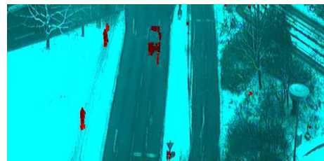
Figure 2: Colour sequence. Detection of moving objects (in red) based on the statistics of the difference of the colour pixels with the median image of the sequence (sequence dtneu-winter).
