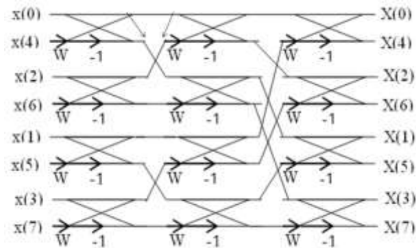
Figure 9: Flow Diagram of FFT using Multiplier-less Technique
