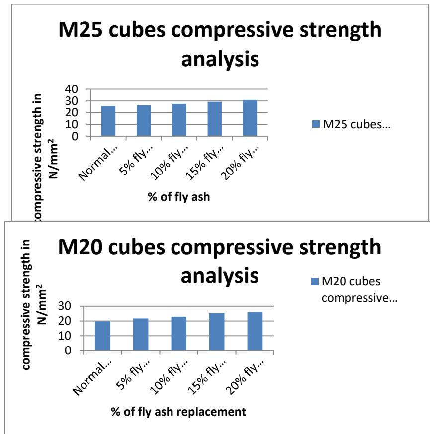
1. The compressive strength of M20 grade of concrete increase with increase in fly ash content. Increase in compressive strength of concrete at the age of 28 days was found to be 1.674% with 5% fly ash, 2.903% with 10% fly ash and when we added admixture with 15 and 20% fly ash compressive strength increases rapidly like 5.244% for 15%, and 6.104 for 20% replacement of cement with fly ash.
