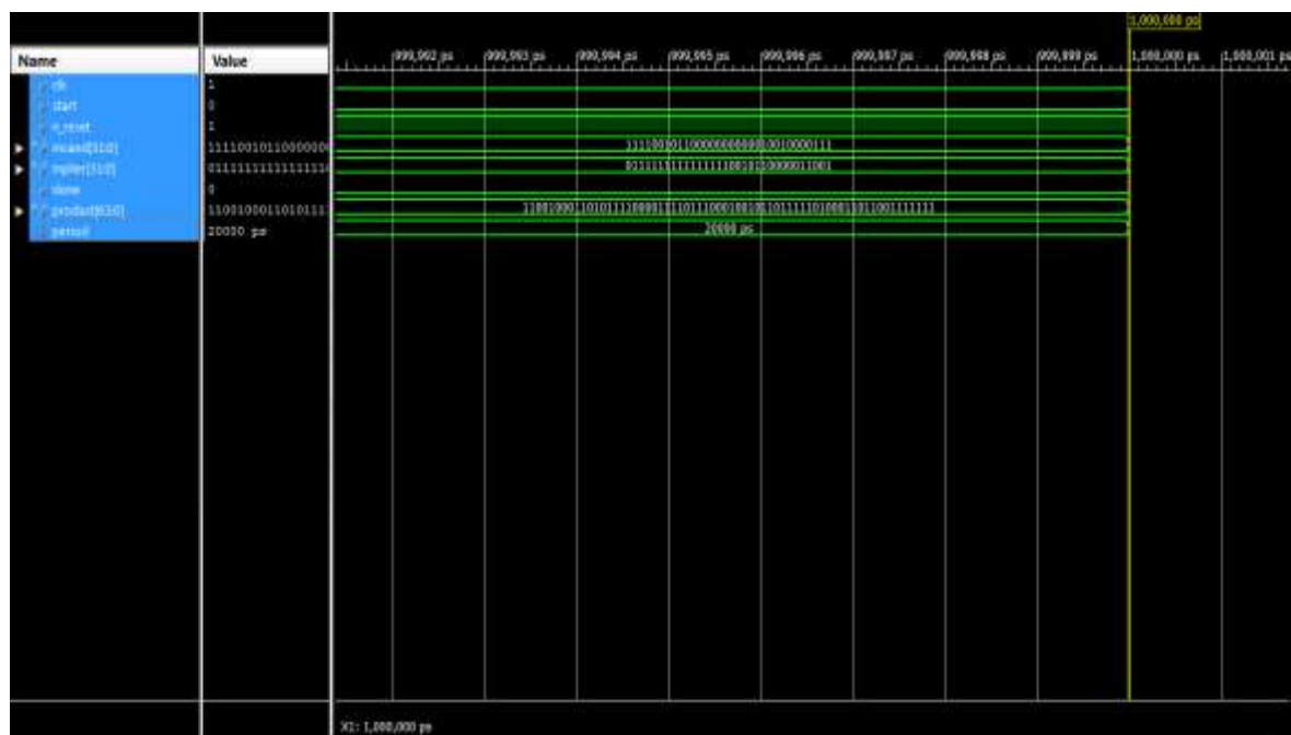
Figure 10 Clock representation of micro-pipelined 32-bit multiplier
