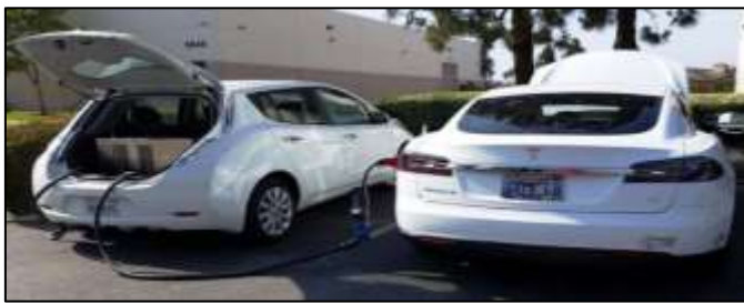
Figure 11. A Nissan Leaf is transferring energy to a Tesla Model S through a conductive charging cable [4].
