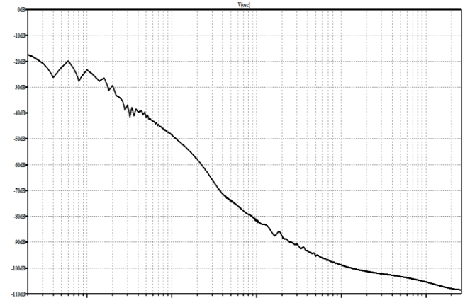
Figure 6 FFT plot for VCO using simple inverter
