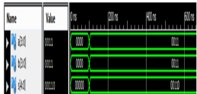
Fig. 10: VHDL Test Bench of 4-bit BK Adder
