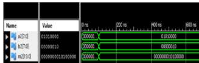
Figure 10: Output Waveform of the 8-bit Vedic Multiplier
