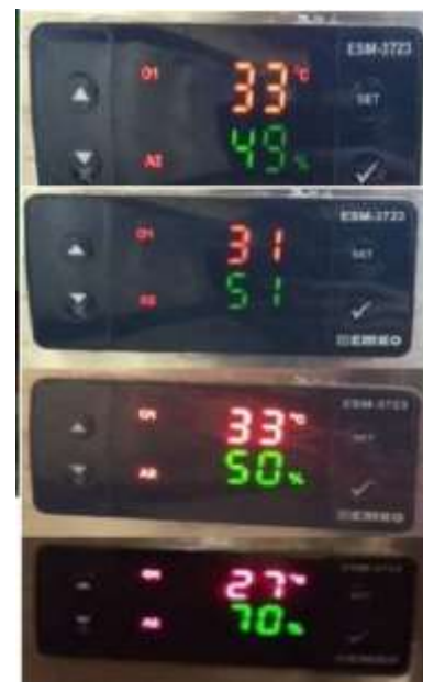
Figure No.10- Temperature and humidity percentage display on LED.
