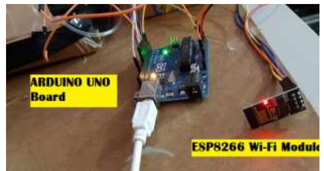
Figure.4: Shows ESP8266 Wi-Fi connections with Arduino Uno board
