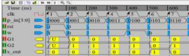
Figure 7: Output Waveform of 4-bit Serial in Parallel out Shift Register
