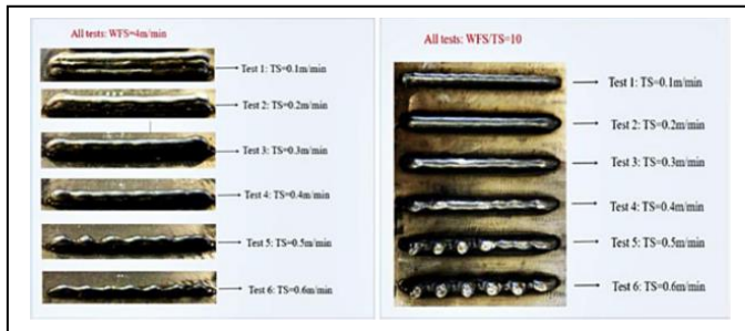
Fig. 3. Single bead deposition with different torch speed.
