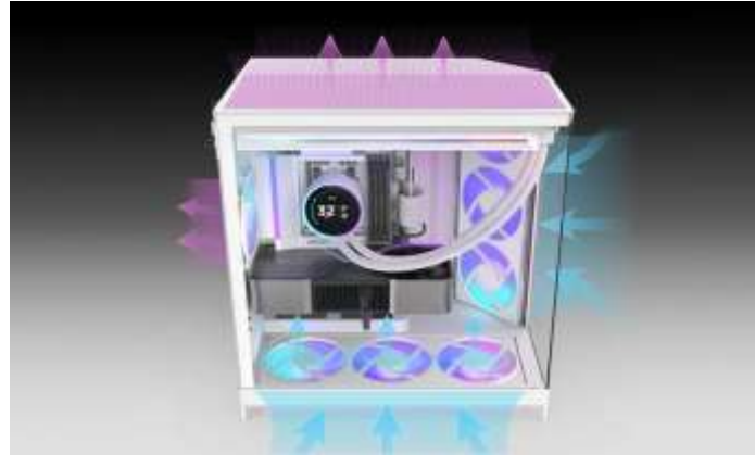
Figure 1: Airflow and Thermal Management Inside Gaming PC Cabinet (digitaltrends.com)
