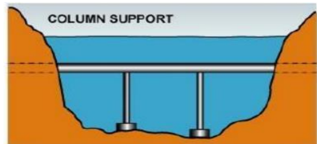
Fig. 3(b): SFT supported on columns
