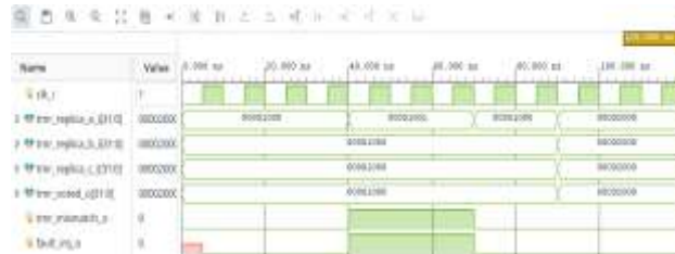
Figure 5.5: XSim behavioral simulation of selective-TMR fault masking showing single-replica corruption, majority-voted output retention, mismatch detection and fault indication
