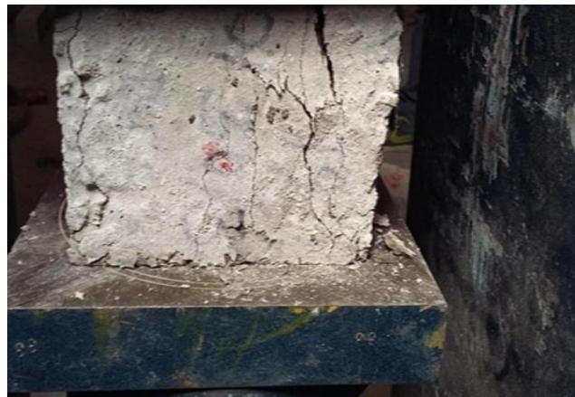
Fig. 2: Compressive Strength Testing
