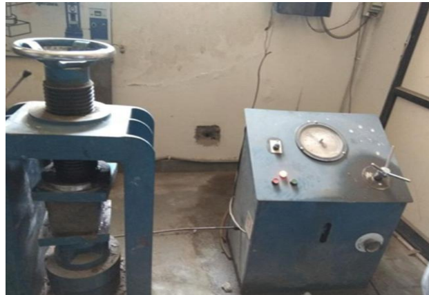
Fig. 1: Compressive Strength Testing Machine
