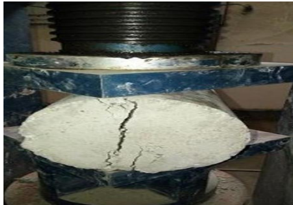
Fig. 4: Split Tensile Strength Testing of Cylinder
