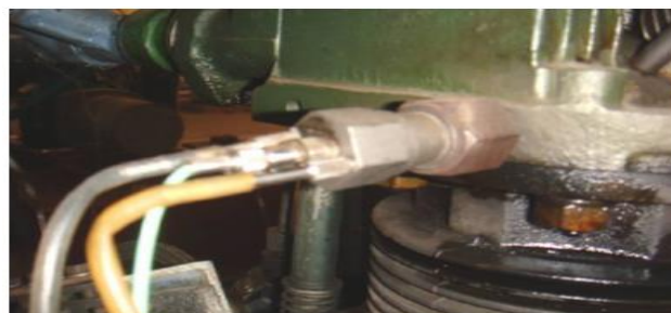
Figure 2: Photographic view of pressure transducer fitted in the cylinder head
