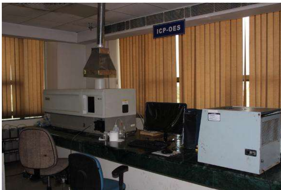
Figure 1: Inductively Coupled Plasma–Optical Emission Spectroscopy (ICP–OES) Instrument used for elemental analysis of water samples.
