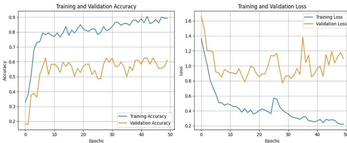
Fig. 6 — ConvNeXt Model Training Curves Training and Validation Accuracy / Loss — ConvNeXt Transfer Learning Baseline
