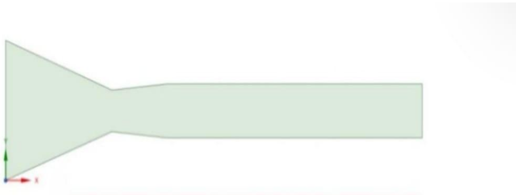
Figure 2: Two-dimensional CFD model of the nozzle for Mach number 2
