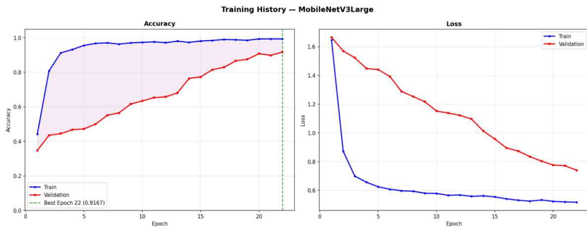
Fig. 5. Training History — MobileNetV3Large: Accuracy (left) and Loss (right) curves over 22 epochs showing training (blue) and validation (red) progression.
