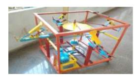
FOUR-WAY HACKSAW MACHINE BY USING RADIAL CRANK MECHANISM
